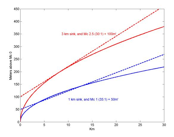
[FIGURE CAPTION KEEP WITH FIGURE] Figure 1. Safety glides, with 2% chance of not making it.
